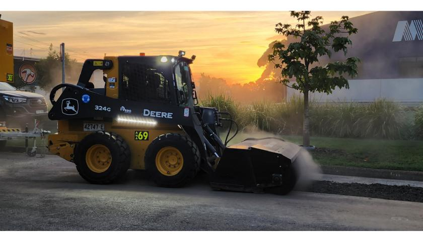
The ShoulderMaster Sweeper Broom is a tough, reliable, and easy-to-use open-face broom. It features a large collection bucket with bolt-on wear plates for easy maintenance. The brush is adjusted with an easy and quick 4-stage adjuster bolt with total brush replacement exchanged by a one-piece poly brush for easy on-site maintenance.
